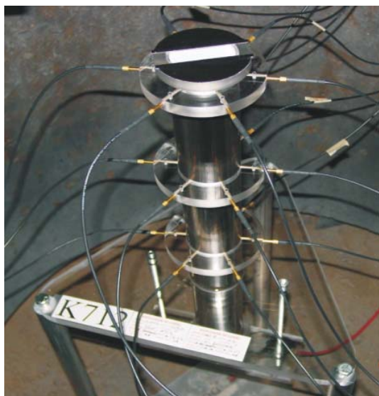
Fig. 4 Cylinder test, where the detonation runs upward. The three pins rings are visible as is the end slit for breakout. The laser beam for wall velocity will hit the copper about two thirds of the way up. The cylinder sits inside a shrapnel catcher inside the 1.0 kg shot tank
